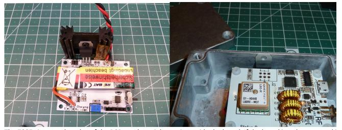
The 7805 sits near the edge of the PCB so a heatsink can sit outside the board. If the board is to be mounted in a metal box then the case of the box can be used as a heatsink.
