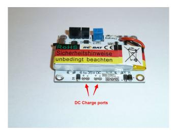
Max voltage on the input is 35Volt but as stated before, higher voltages will heat up the regulator
