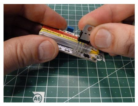
Insert the legs as long as is suitable in your situation and solder the three pins on the bottom side of the board.
