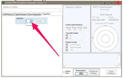
Next, plug in the USB cable from the transmitter to the computer and click the chevron again to see the list of available serial ports.
