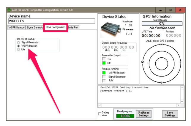
Once this setting is saved, the transmitter can be unplugged from the computer and be powered from another power source. It will run continuously 24/7 as long as it has a GPS fix.
