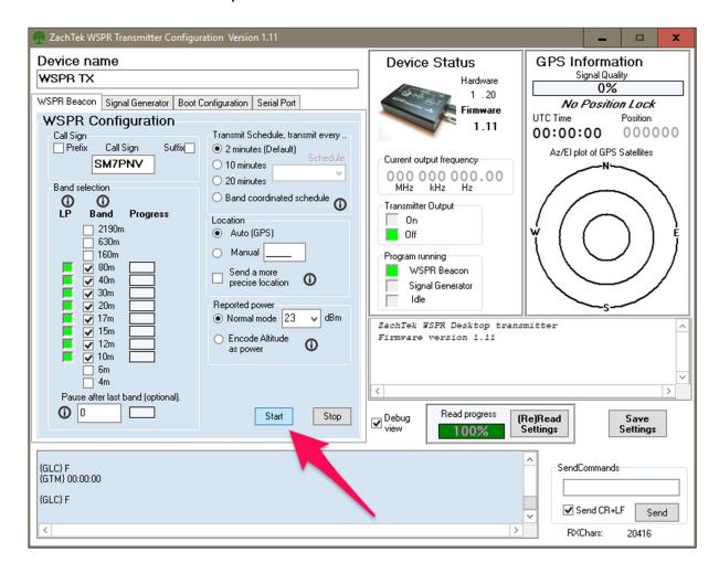
K. Once the WSPR mode has been started it will continually transmit the WSPR beacon on all bands that are enabled. If you change something in the software while the beacon is running it, will temporary drop out of WSPR beacon mode to handle the new setting. It will then go back in to beacon mode again.
