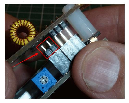
Align the pin header with the pins and Insert the boards together.
