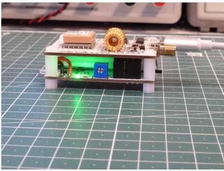
The blue potentiometer sets the charge current. Turn it fully clockwise to charge with up to 1 Ampere. Counter-clockwise to set charge current to 100mA If you want to use the optional DC inputs to charge the LiPo you will need to solder in the 7805Voltage regulator.
