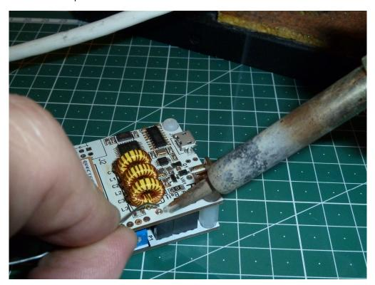
Screw in the plastic hex studs fasteners that came with the LiPo board. \\
