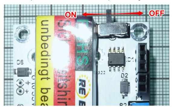
Make sure that the 2-pole female pin header on the LiPo board has its male pin header inserted in it. This is usually the case when it comes delivered so just verify it is there.
