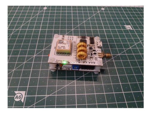
If a USB cable is inserted to the mated board it will charge the LiPo battery. The charging circuit on the board will automatically turn on or off the charging when necessary. The protection circuits will disconnect the battery if it gets fully depleted
